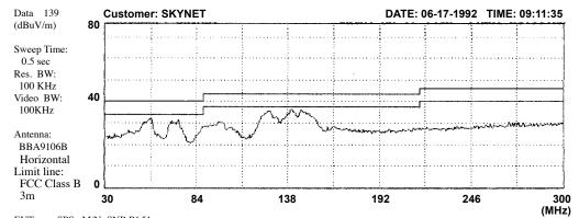
EUT : SPS. M/N: SNP-PA51 Power : 120Vac, 60Hz Memo : CHAMBER, 8568B Spectrum Analyzer
