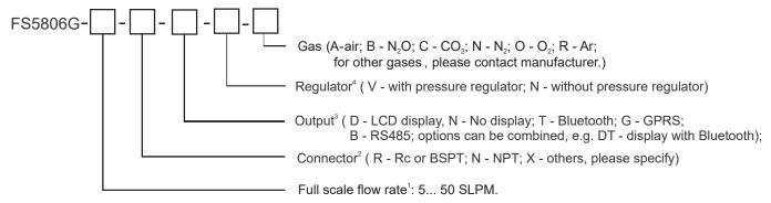
1. Numerical maximum flow rate only, for example, 50 meaning full scale flow rate of 50SLPM.
