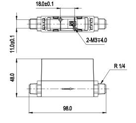
The outer mechanical dimensions for both 3mm and 8mm flow channel are identical. The standard BSPT/Rc threaded adapters can be fully replaced by customized ones.
