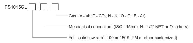
1. Numerical only, customizable flow rate shall be within 100 ~ 180 SLPM.
