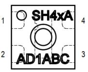
**Figure 13** Pin assignment (transparent top view). Dashed lines are only visible if sensor is viewed from below. The die pad is not directly connected to any pin.
