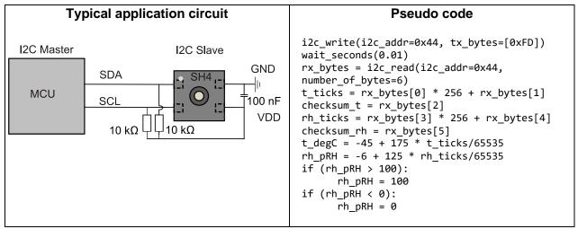
**Figure 1:** Typical application circuit (left) and pseudo code (right) for easy starting with the I2C interface. For details on the signal cropping in the last four lines see **section 4.6**.
