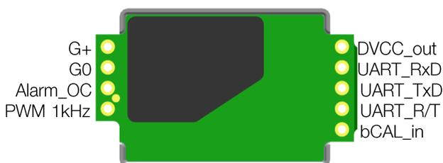
Figure 2. Pin assignment
