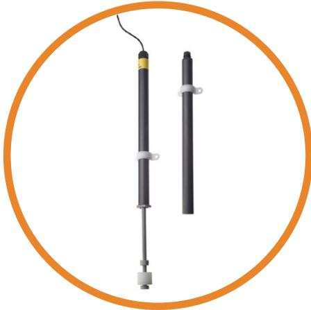
A vertical float switch, with either normally open or normally closed switch action, permanently joined to a 300mm PVC tube. This provides a switch, whose overall switching depth can be varied between 123mm and 423mm
