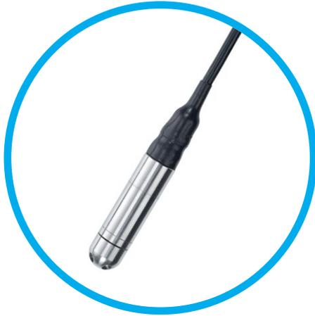
The ILTS is designed for use in continuous submersion in liquids such as water, oil and fuels. The probe uses the latest piezo-resistive media-isolated silicon sensing technology and a stainless steel diaphragm. Housed within a 316L stainless steel, or high grade Duplex stainless steel housing, this submersible transmitter is the ideal product for hydrostatic level measurement where temperature is also a critical part of the measurement.
