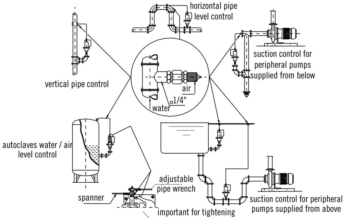
FCNMAS type applications - solution suitable only for pressurised tubing
