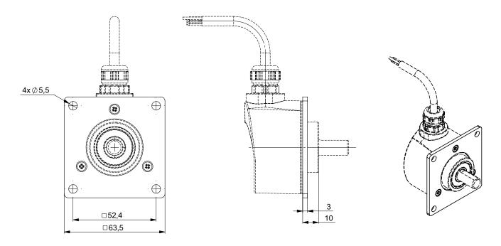
AH05\_14 Standard clamping, Connection BJR (Radial Cable), coupling 9445/012 mounted on the body
