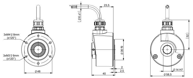
AH05S14/0M/ Flange side clamping, Connection BFR (Radial M12)
