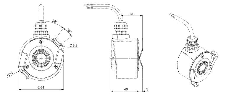
AH05\_14 Standard clamping, Connection BJR (Radial Cable), coupling 9445/015 mounted on the body
