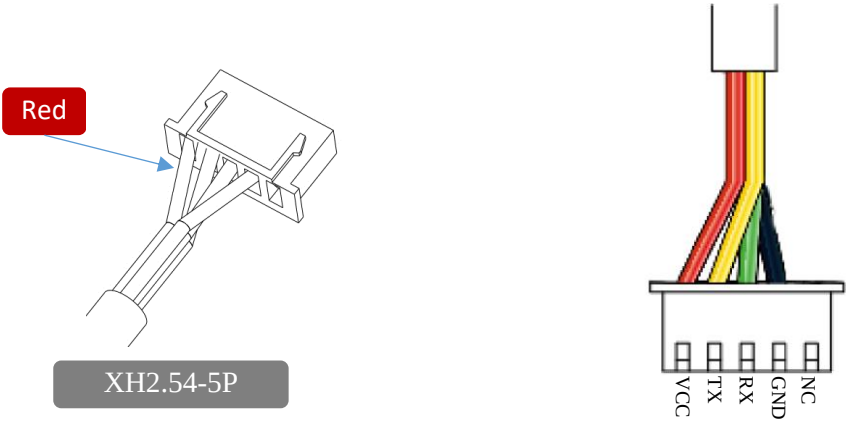
Figure 2-5 RPLIDAR Power Interface Definition
