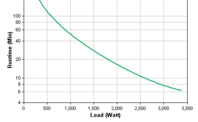
Curve fit to measured runtime data. All measurements taken with new, fully charged batteries, at
