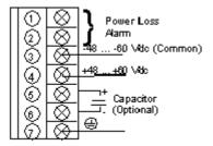
NOTE: A normally closed relay contact rated at 220 Vac, 6A / 30 Vdc, 5A is available on terminals 1 and 2 of the power terminal strip. This contact set may be used to signal input power OFF, or a power supply failure.
