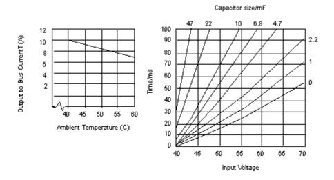
NOTE: Tolerance to input interruptions may be increased by adding a  $\geq$  80 Vdc electrolytic capacitor between 5 and 6 of the power terminal strip. Refer to the hold-up capacitor timing chart (above) for capacitor values.
