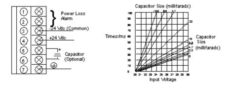
NOTE: A normally closed relay contact rated at 220 Vac, 6A / 30 Vdc, 5A is available on terminals 1 and 2 of the power terminal strip. This contact set may be used to signal input power OFF, or a power supply failure. The relay will de-energize when input power drops below 8 Vdc.
