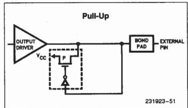
**Figure Bb. Bus Hold Circuitry Pins 4-6, 68**
