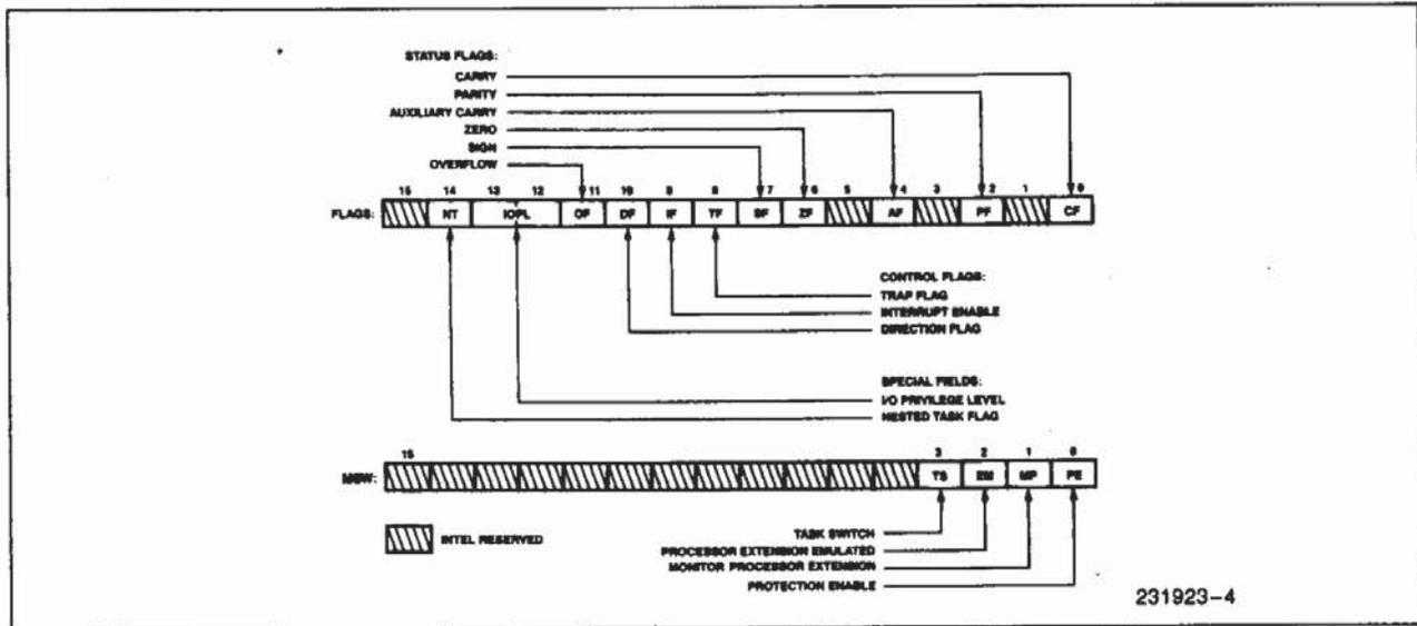
Figure 3a. Status and Control Register Bit Functions
