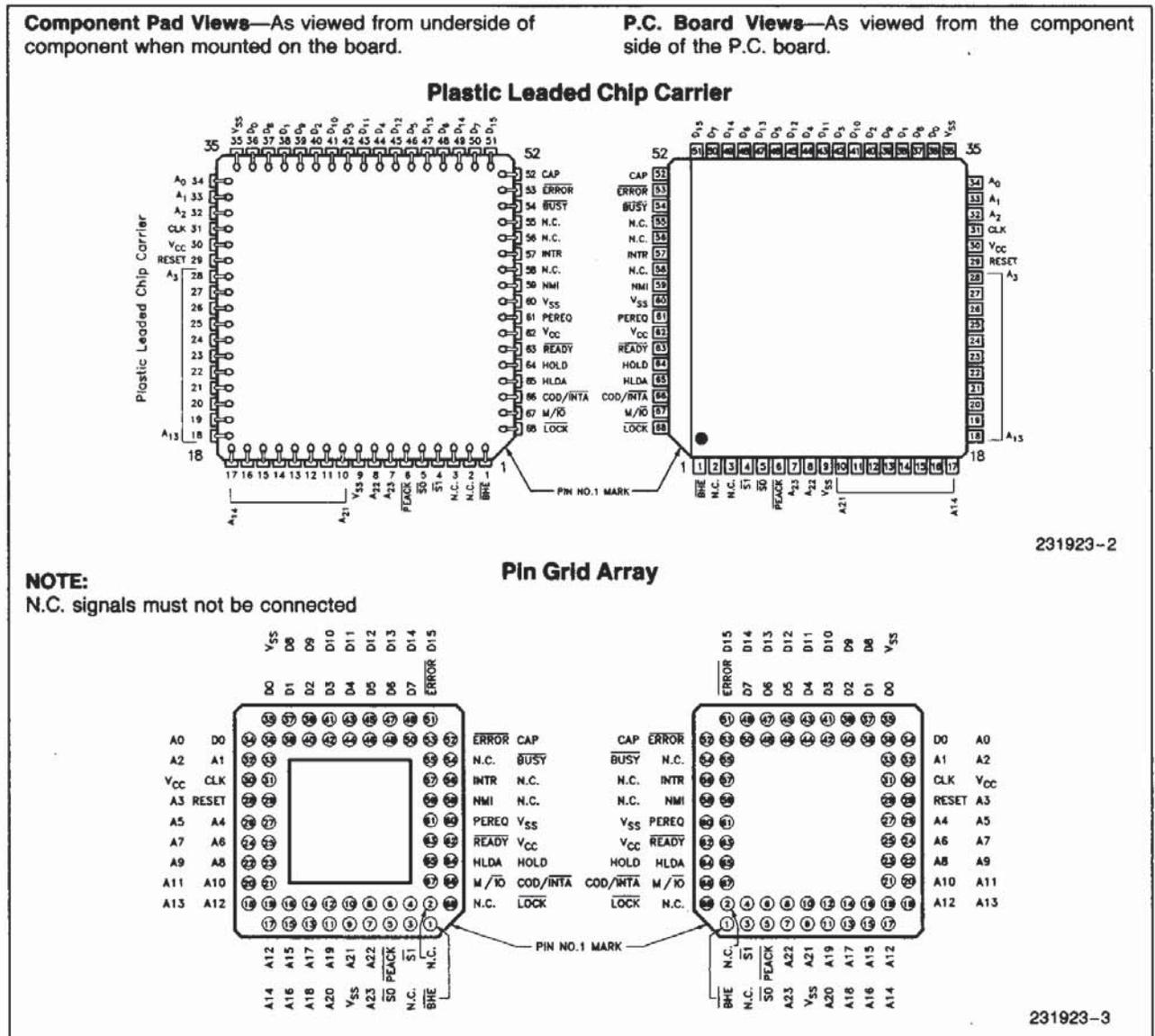
**Figure 2. 80C286 Pin Configuration**
