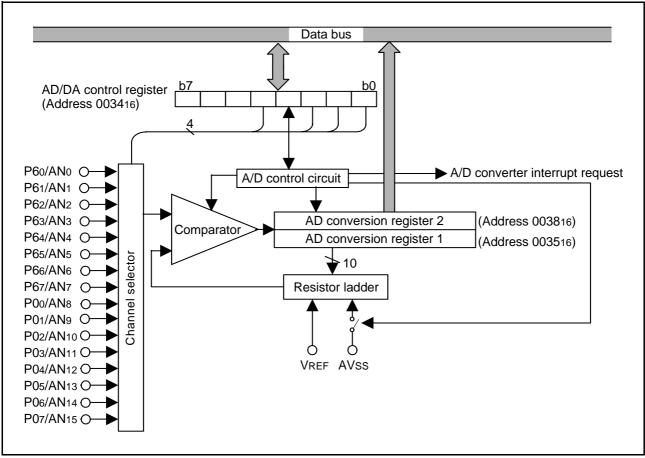
Fig 55. Block diagram of A/D converter
