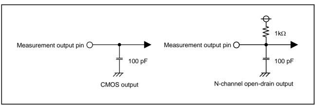
Fig 100. Circuit for measuring output switching characteristics
