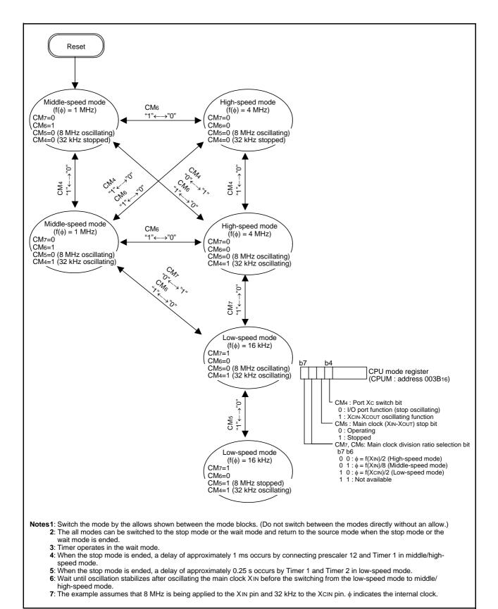
Fig 66. State transitions of system clock
