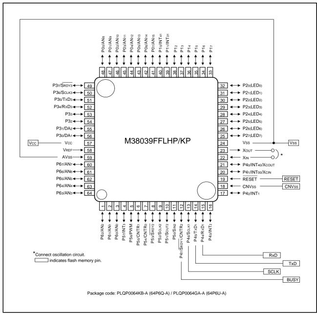
Fig 77. Connection for standard serial I/O mode 1 (M38039FFLHP/KP)
