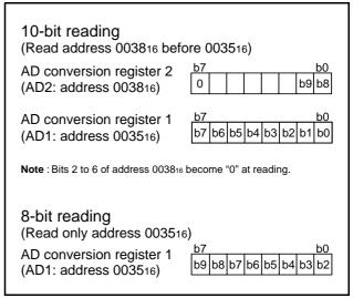
Fig 54. Structure of 10-bit A/D mode reading
