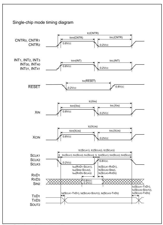
Fig 101. Timing diagram (in single-chip mode)
