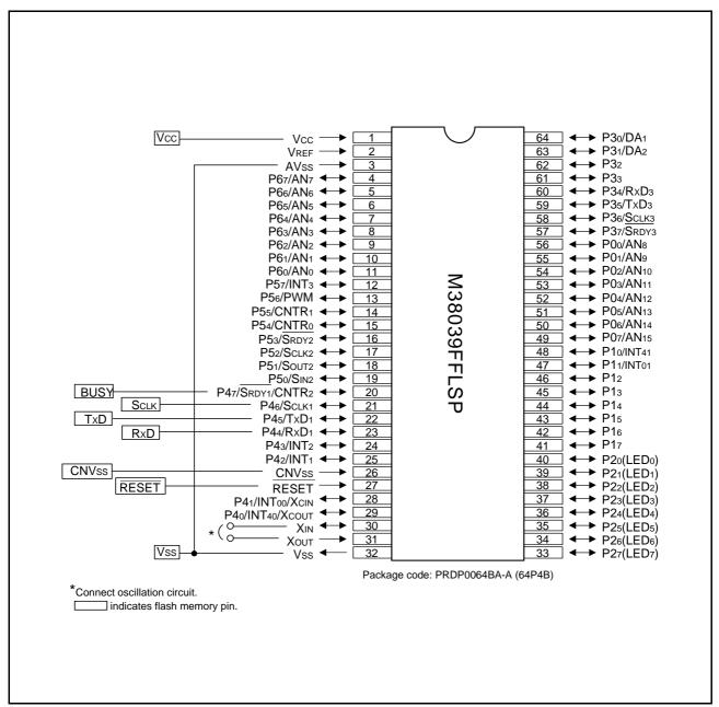
Fig 79. Connection for standard serial I/O mode 1 (M38039FFLSP)
