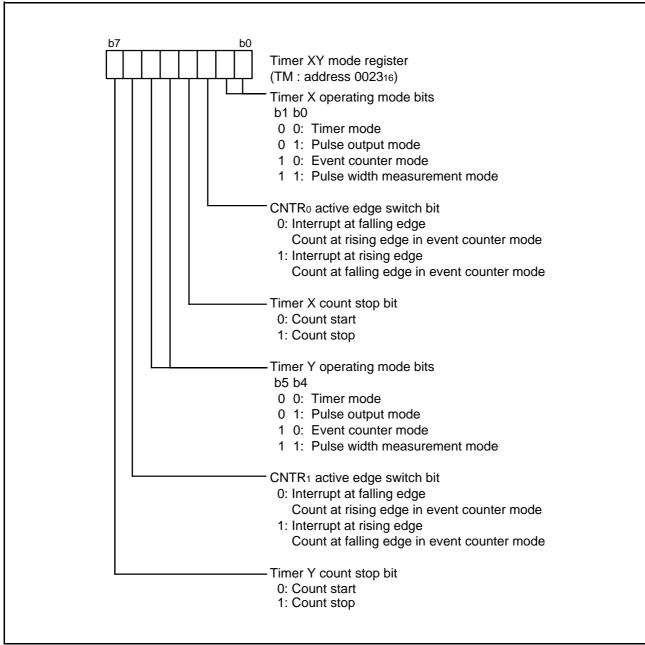
Fig 26. Structure of timer XY mode register
