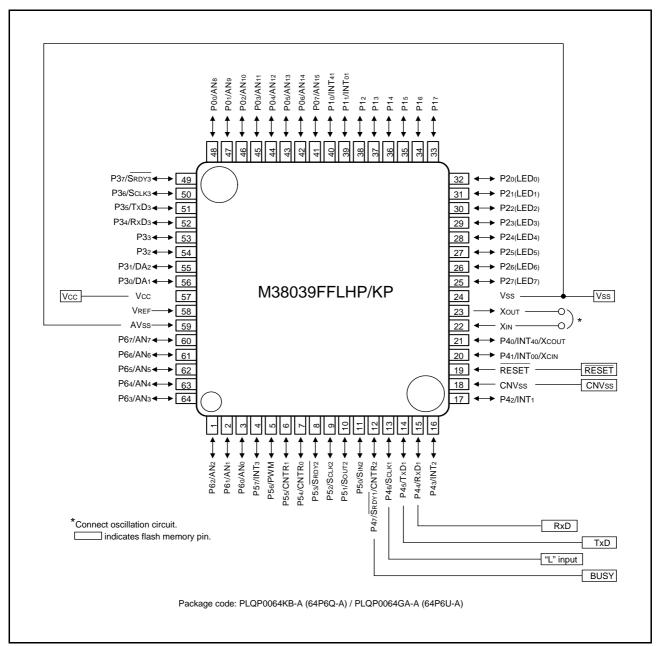
Fig 78. Connection for standard serial I/O mode 2 (M38039FFLHP/KP)
