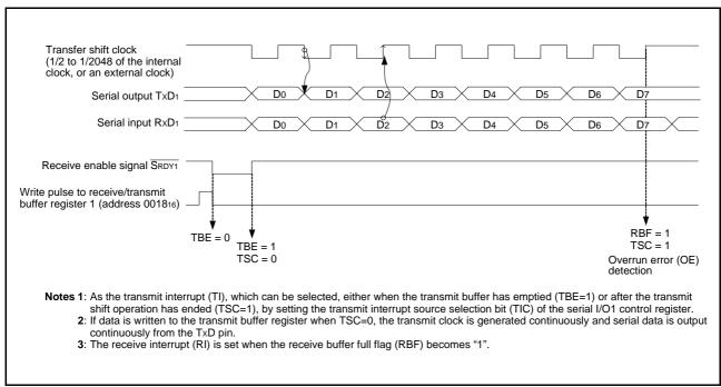
Fig 37. Operation of clock synchronous serial I/O1
