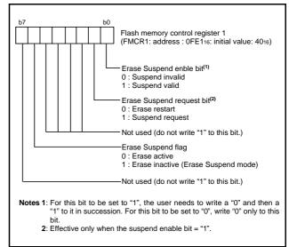
Fig 69. Structure of flash memory control register 1
