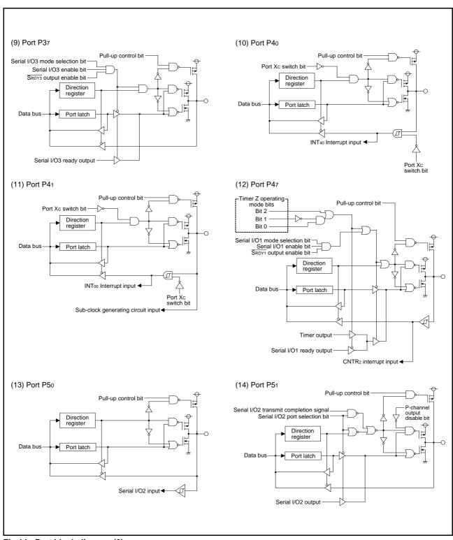
Fig 14. Port block diagram (2)
