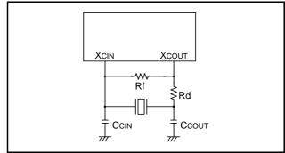
Fig 98. Ceramic resonator circuit
