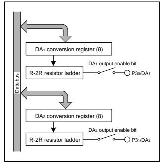
Fig 56. Block diagram of D/A converter
