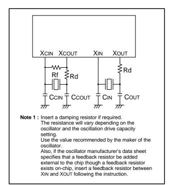
Fig 63. Ceramic resonator circuit
