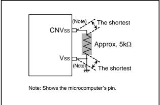
Fig 94. Wiring for the CNVss
