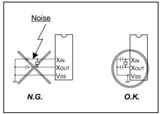
Fig 91. Wiring for clock I/O pins
