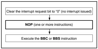
Fig 96. Sequence of check of interrupt request bit
