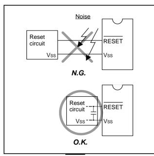
Fig 90. Wiring for the RESET pin
