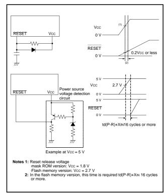
Fig 60. Reset circuit example
