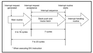
Fig 22. Time up to execution in interrupt routine
