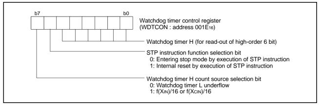
Fig 59. Structure of Watchdog timer control register
