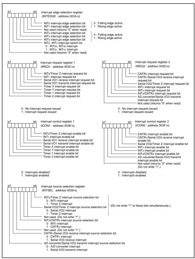
Fig 21. Structure of interrupt-related registers
