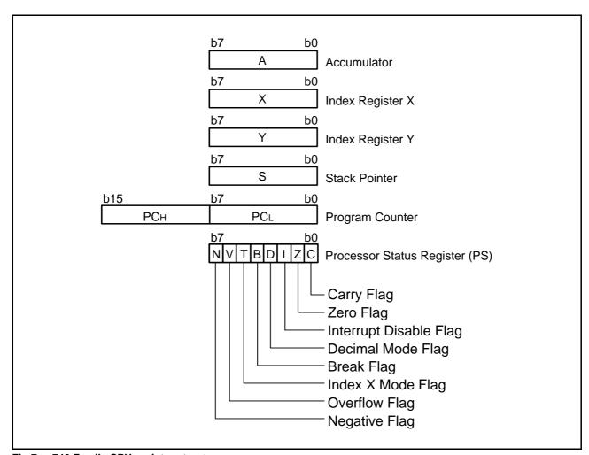
Fig 7. 740 Family CPU register structure
