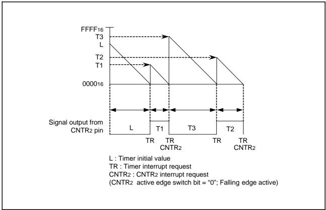
Fig 34. Timing chart of programmable waveform generating mode
