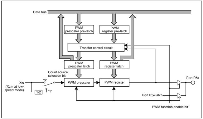
Fig 50. Block diagram of PWM function
