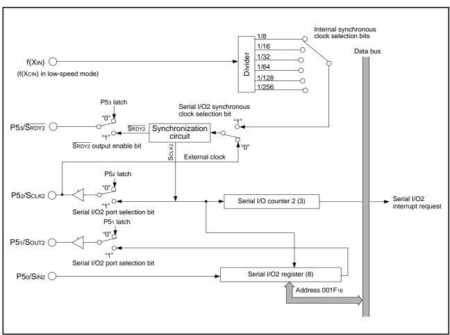
Fig 42. Block diagram of serial I/O2
