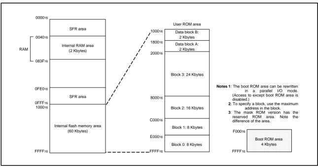
Fig 67. Block diagram of built-in flash memory
