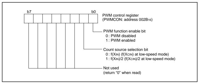
Fig 51. Structure of PWM control register
