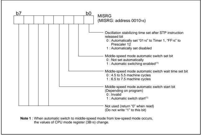
Fig 10. Structure of MISRG
