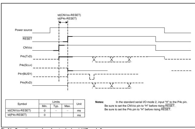
Fig 84. Operating waveform for standard serial I/O mode 2
