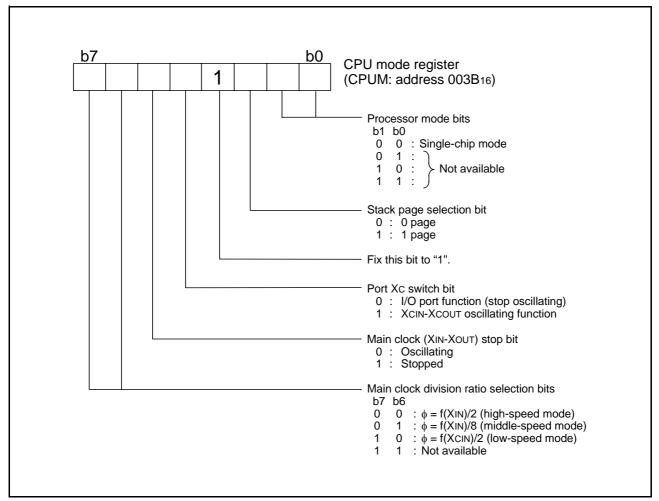
Fig 9. Structure of CPU mode register
