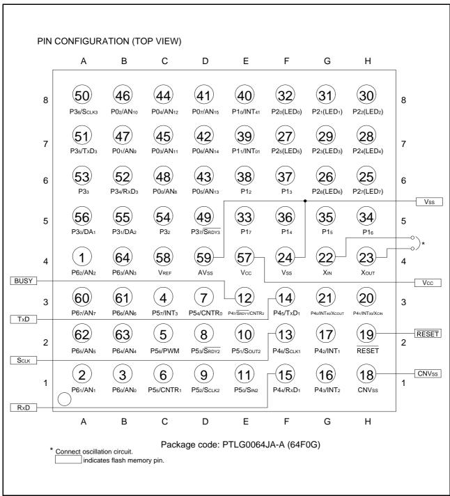
Fig 81. Connection for standard serial I/O mode 1 (M38039FFLWG)
