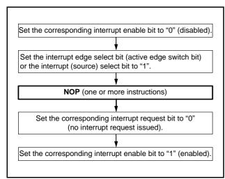
Fig 95. Sequence of changing relevant register
