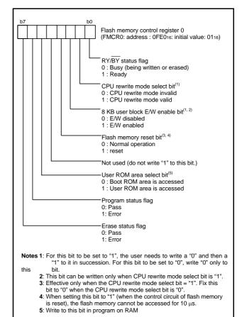
Fig 68. Structure of flash memory control register 0
