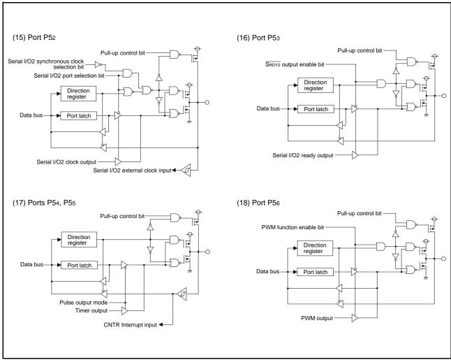
Fig 15. Port block diagram (3)
