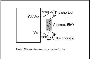
Fig 99. Wiring for the CNVss
