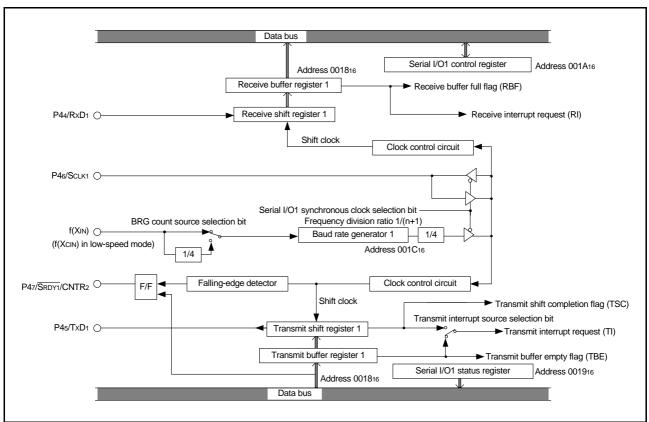
Fig 36. Block diagram of clock synchronous serial I/O1
