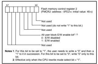
Fig 70. Structure of flash memory control register 2
