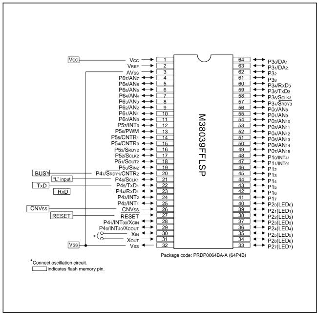
Fig 80. Connection for standard serial I/O mode 2 (M38039FFLSP)
