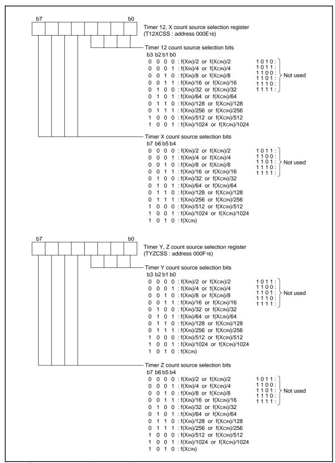
Fig 27. Structure of timer 12, X and timer Y, Z count source selection registers
