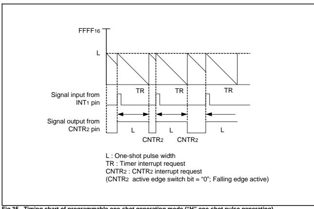
Fig 35. Timing chart of programmable one-shot generating mode ("H" one-shot pulse generating)
