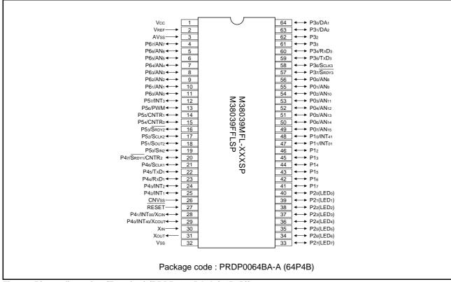
Fig 2. Pin configuration (Top view) (PRDP0064BA-A (64P4B))
