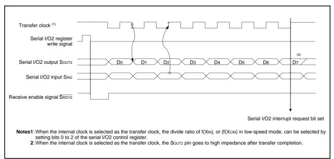
Fig 43. Timing of serial I/O2
