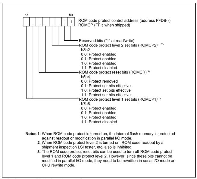
Fig 75. Structure of ROM code protect control address
