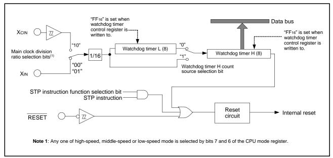
Fig 58. Block diagram of Watchdog timer
