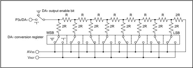
Fig 57. Equivalent connection circuit of D/A converter (DA1)
