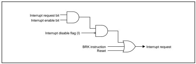
Fig 20. Interrupt control diagram
