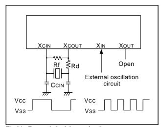
Fig 64. External clock input circuit
