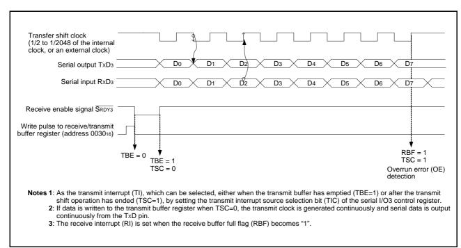
Fig 45. Operation of clock synchronous serial I/O3
