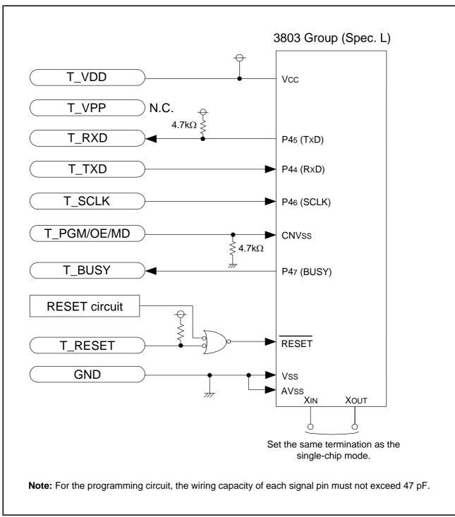
Fig 85. When using programmer (in standard serial I/O mode 1) of Suisei Electronics System Co., LTD, connection example
