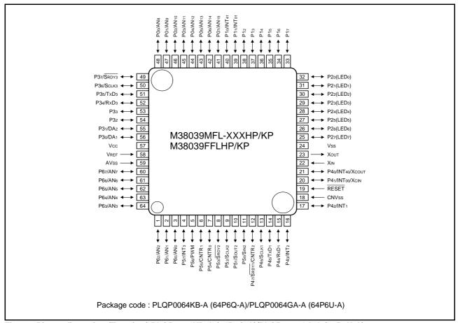
Fig 1. Pin configuration (Top view) PLQP0064KB-A (64P6Q-A)/PLQP0064GA-A (64P6U-A)
