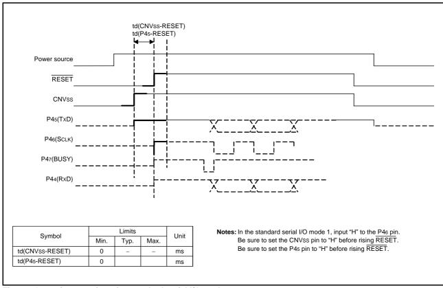
Fig 83. Operating waveform for standard serial I/O mode 1
