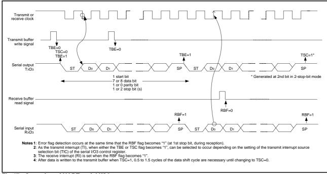
Fig 47. Operation of UART serial I/O3
