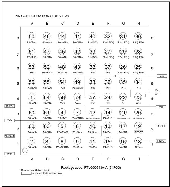
Fig 82. Connection for standard serial I/O mode 2 (M38039FFLWG)
