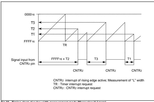
Fig 33. Timing chart of pulse width measurement mode (Measuring "L" term)
