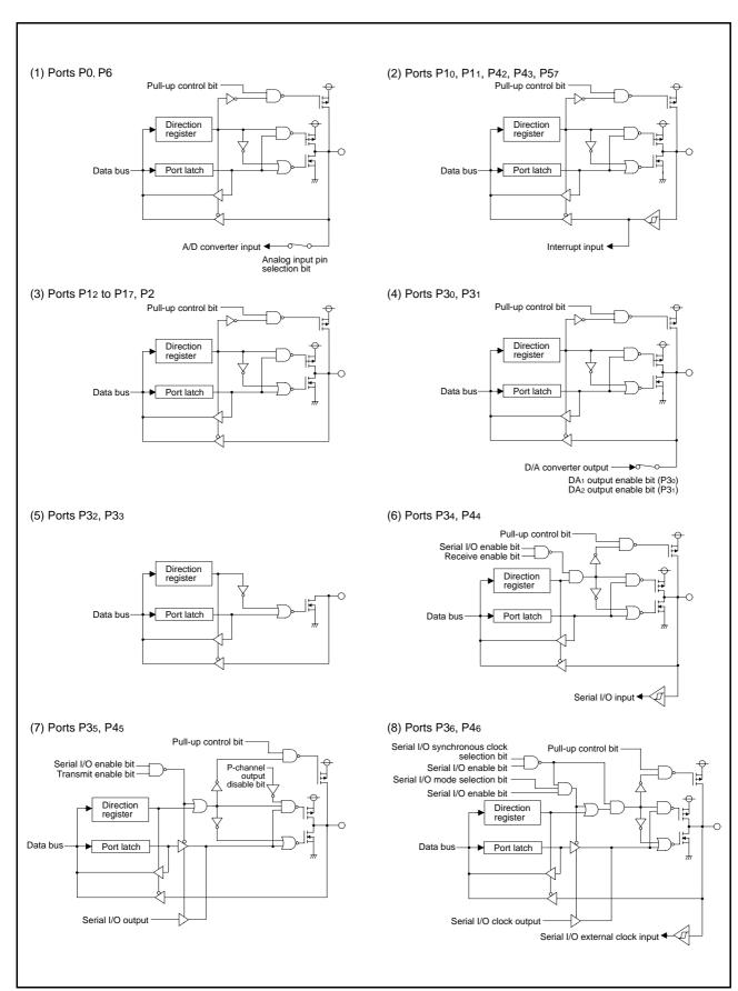
Fig 13. Port block diagram (1)
