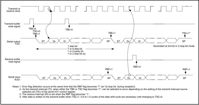
Fig 39. Operation of UART serial I/O1
