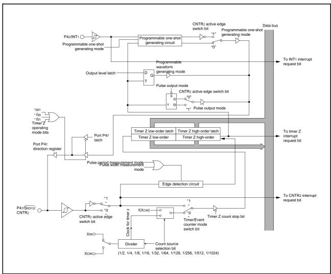
Fig 28. Block diagram of timer Z
