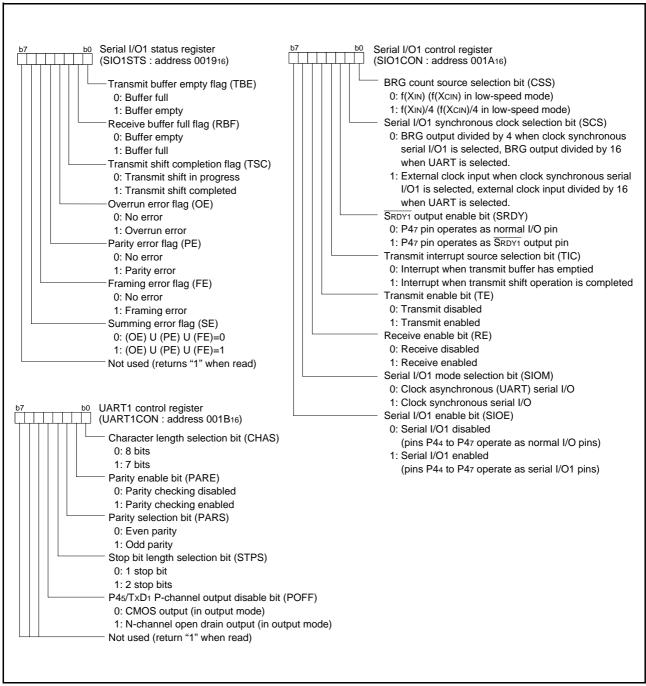
Fig 40. Structure of serial I/O1 control registers
