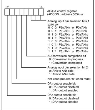
Fig 53. Structure of AD/DA control register
