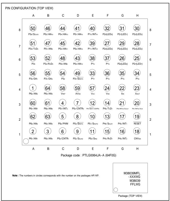
Fig 3. Pin configuration (Top view) (PTLG0064JA-A (64F0G))
