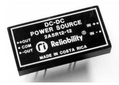
These 2 Watt regulated DC/DC converters operate from an input of 5 volts and make available at board level dual outputs of  $\pm 12$  or  $\pm 15$  VDC. They operate without derating or heatsinking over the full temperature range. Solid tantalum capacitors are used for enhanced reliability. The units are designed for analog applications such as Op Amps, A/D, D/A and F/V converters. They can also be used for negative voltage bias applications.
