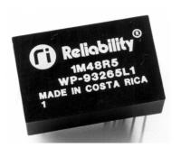
These 1 and 1.5 Watt DC/DC converters operate from a nominal 48v source and make available isolated single 5v and dual 5v outputs at the board level. The converters operate without derating over their full temperature range. Solid tantalum capacitors are used for enhanced reliability. Applications include telecommunications and industrial controls where space is at a premium.
