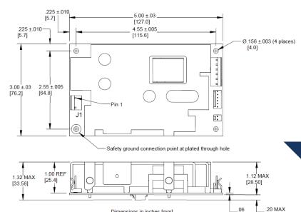
Note: Recommended standoff size is .375" high and all mounting hardware should be less than .28" in diameter. A standoff less than .375" high is acceptable when a thin insulator, 0.4mm thick (polyester, fish paper or equivalent UL rated 94V-2 minimum) is placed between the XR160 and the mounting chassis (refer to applicable UL standard for clearance requirements).
