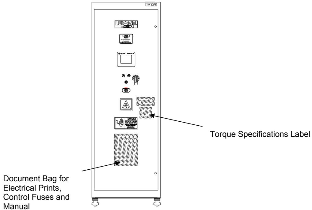
**Figure 15: Location of Torque Specifications Label**
