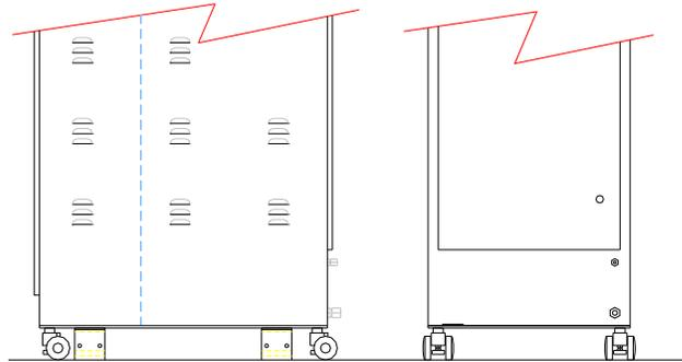
**Figure 8: Seismic Brackets (top-half) Attached to Cabinet**
