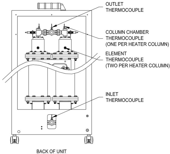
**Figure 43: Thermocouple Locations**
