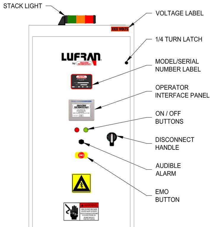
Figure 17: Front Panel Layout
