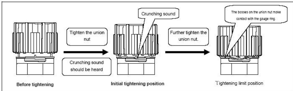
**Figure 13: Super 300 type Pillar fittings tightening procedure**
