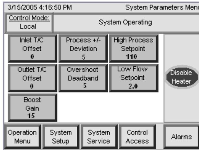
**Figure 23: System Parameters Menu Screen**
