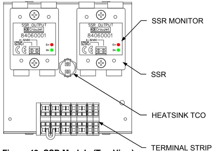
**Figure 48: SSR Module (Top View)**
