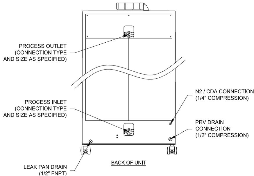
**Figure 10: Water, Gas Plumbing Connections**
