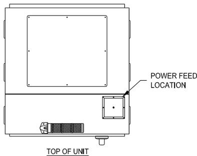
**Figure 14: Electrical Access Panel**
