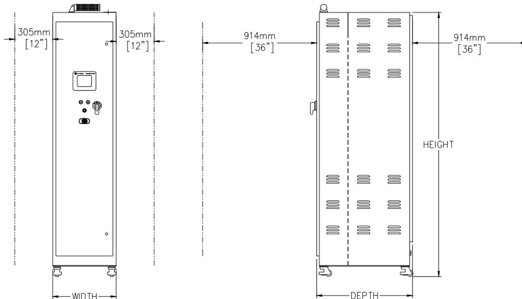
**Figure 5: Clearance Dimensions (Single Column 24-72kW Model Shown)**
