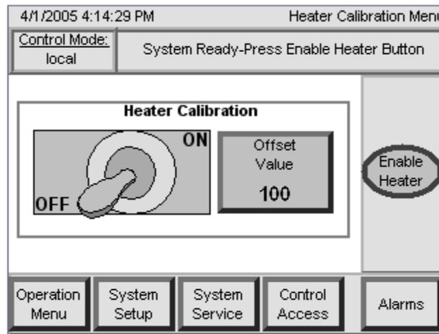
**Figure 25: Heater Calibration Menu Screen**
