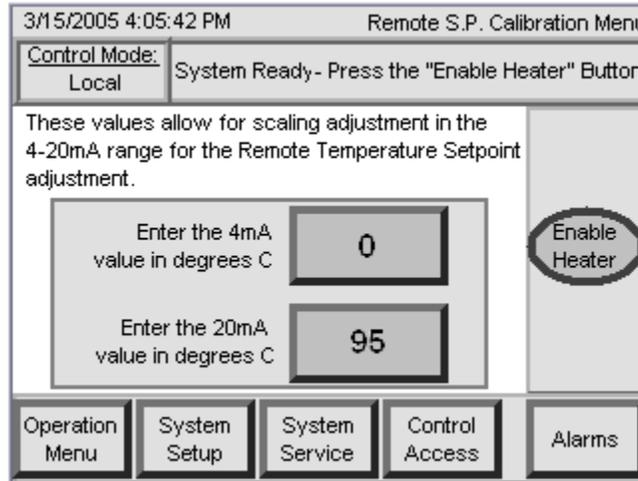
**Figure 26: Remote Setpoint Calibration Menu**
