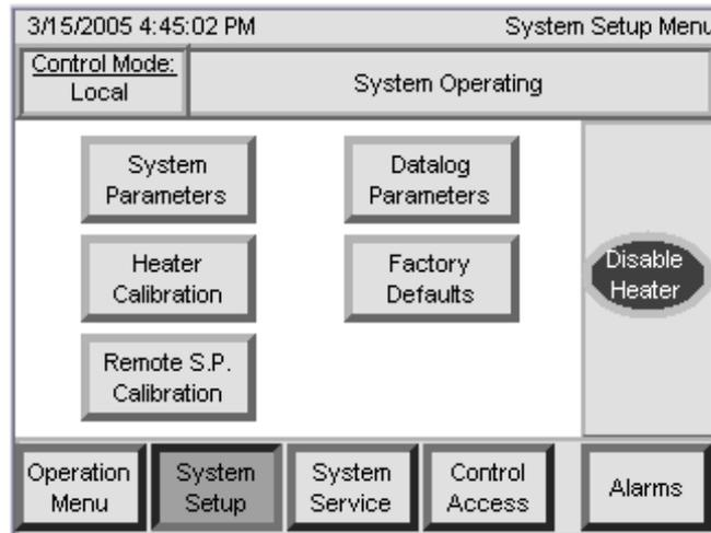
**Figure 22: System Setup Menu Screen**
