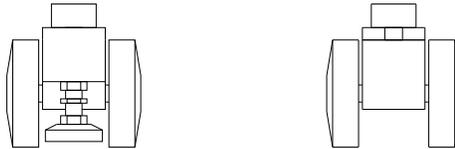
**Figure 7: Leveling Foot Located on Castor**
