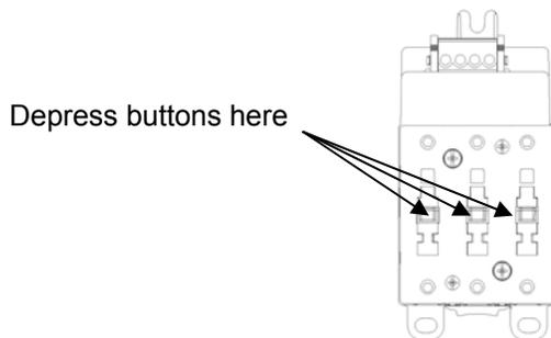
**Figure 51: Safety Contactor**
