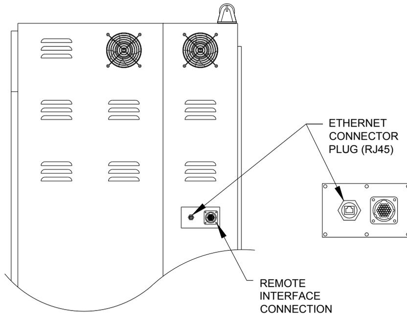
**Figure 40: Ethernet RJ45 connector plug**
