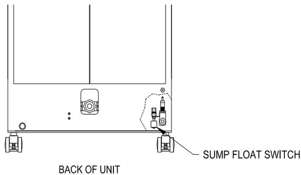
**Figure 44: Leak Detector**
