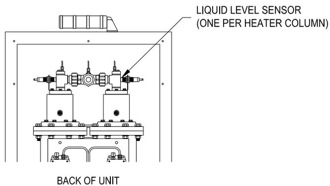
**Figure 42: Liquid Level Sensor**
