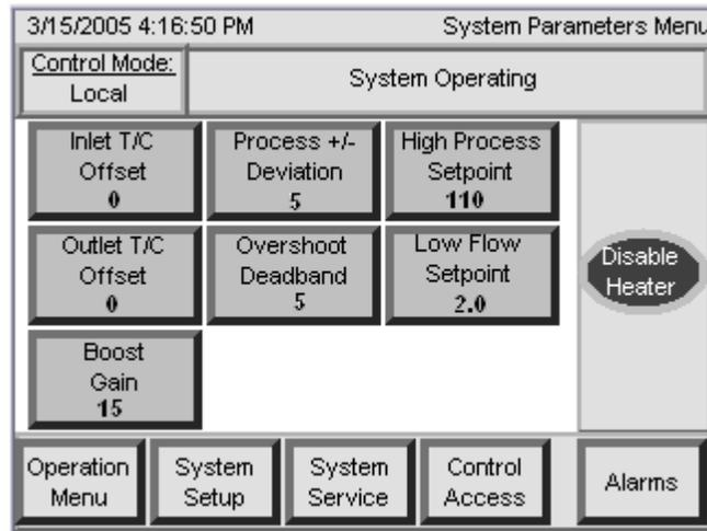
Figure 24: System Parameters Menu Screen
