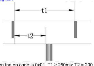
Note: When the op code is 0x01, T1  $\ge$  250ms; T2 = 200  $\sim$  210ms. For op codes 0x10-0x13, T1  $\ge$  90ms; T2 = 65-75ms.
