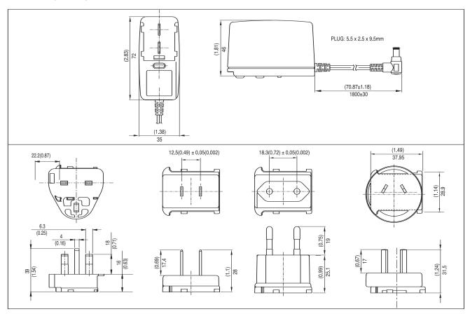
Stock items will be fitted with 5.5x2.5x9.5mm barrel connector, centre positive.
