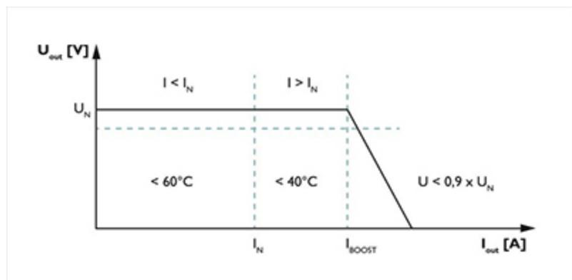
capacitive loads have to be absorbed without voltage dips. With the QUINT Power Boost function a static boost will continuously provide up to 125% of the nominal current. In addition, you can use the dynamic boost to supply up to 150% of the nominal current for 5 seconds when starting up heavy loads.
