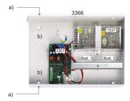
External power supply (3366) inside view: Rectifier (1537) 230 V AC / 24 V DC, Charger board (3367) and space for two batteries, rated 12 V / 6.5-7.5 Ah (size 150 x 65 x 94 mm).
