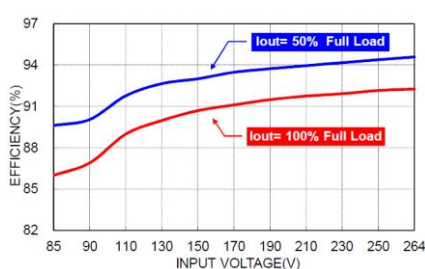
Efficiency vs. Input Voltage MAF300US24 with Forced air cooling
