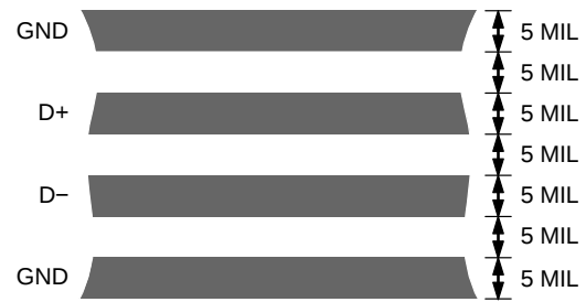
Figure 22. Typical Arrangement of Signal Tracks
