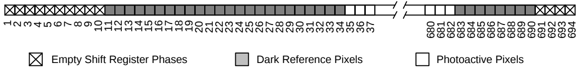
Figure 13. Line Timing Diagram – Single Register Output
