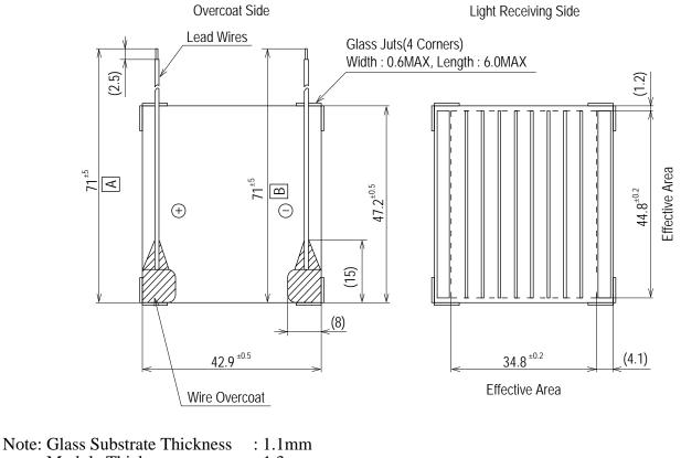
Nodule Thickness1.11mmModule Thickness: 1.3mm maxWire-Overcoat Thickness: 2.5mm max (Including Module)Standard lead wires length: 71mm Marking ( A & B )
