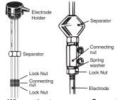
Note: When using two or more Separators, be careful with the mounting direction of the connecting nut screws which connect electrodes. Avoid the screws from touching each other.
