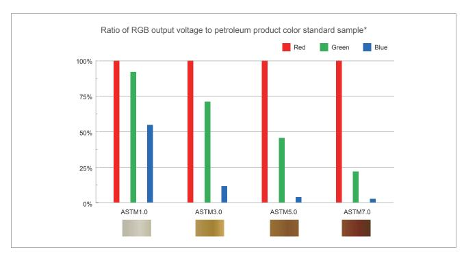
Using the petroleum product color standard sample\*, the output voltage values of the color sensor were graphed as a ratio of green and blue to red.
