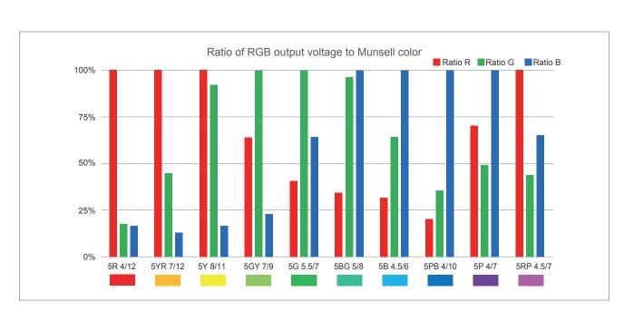
Using Munsell color, the maximum output voltage value of the color sensor was set as 100%, and the ratio of each voltage value to the maximum voltage value was graphed. The ratio of RGB data changes according to the Munsell color.
