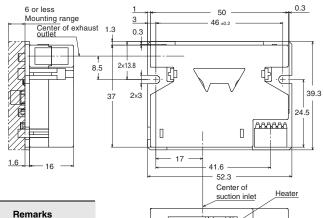
Terminal Pin Remarks name (1) Vcc Input voltage pin V (OUT1) Output voltage pin 1 (2) (3) GND Ground pin (4) Input threshold voltage pin (5) V (OUT2) Output voltage pin 2
