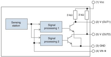
\* For operation, the input threshold voltage Vth must be set to between 0.5 and 3.0 V. The recommended threshold voltage Vth is 0.5 V, which is same detection characteristics for ratings, characteristics and exterior specifications.
