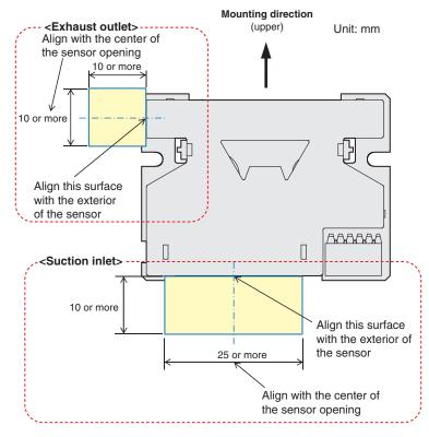
Note1: Ensure that the suction inlet and exhaust outlet are as close to the sensor case
