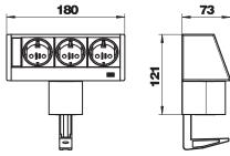
Deskbox with connection cable, cable outlet at the bottom of the profile with a fastening clamp for tabletop thicknesses of 8 to 40 mm.
