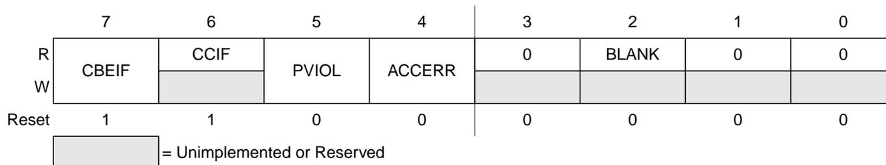
**Figure 2-10. Flash Status Register (FSTAT - Normal Mode)**
