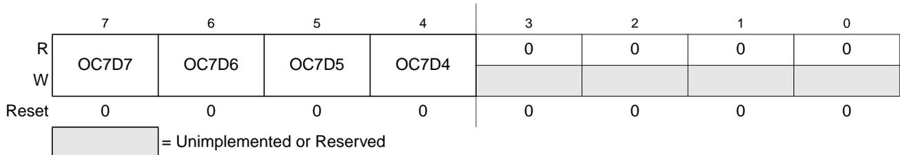
**Figure 13-6. Output Compare 7 Data Register (OC7D)**
