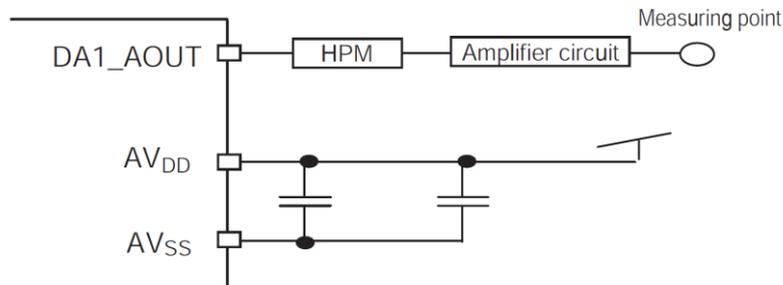
Figure: 5.6 Audio Characteristic Measuring Circuit (a)
