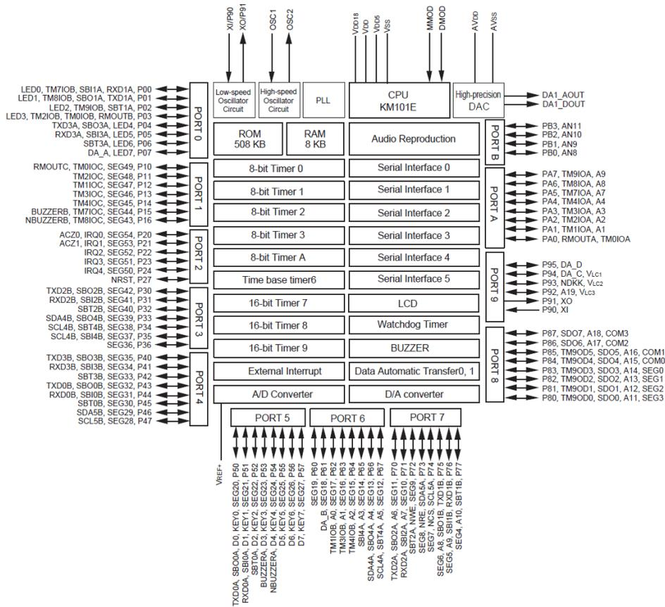
Figure: 4.1 Block Diagram
