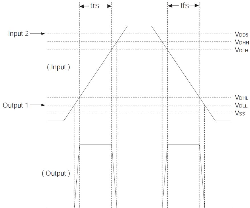
Figure: 5.5 Operation of AC Zero-Cross Detection Circuit
