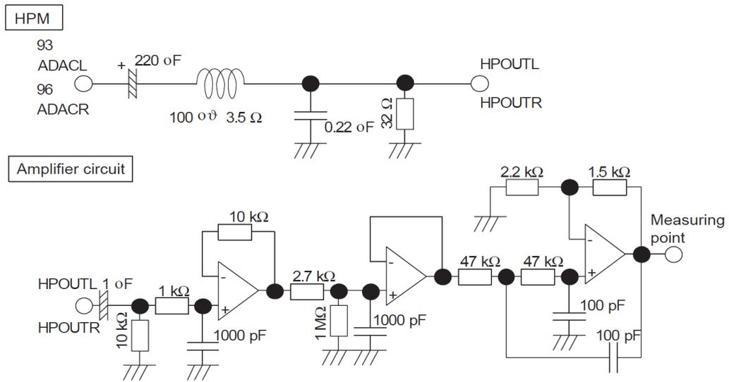
Figure: 5.7 Audio Characteristic Measuring Circuit (b)
