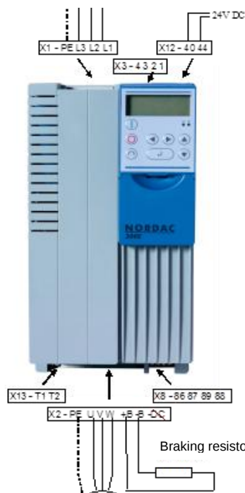
Figure 10: Power connection SK 5xxE up to size 7
