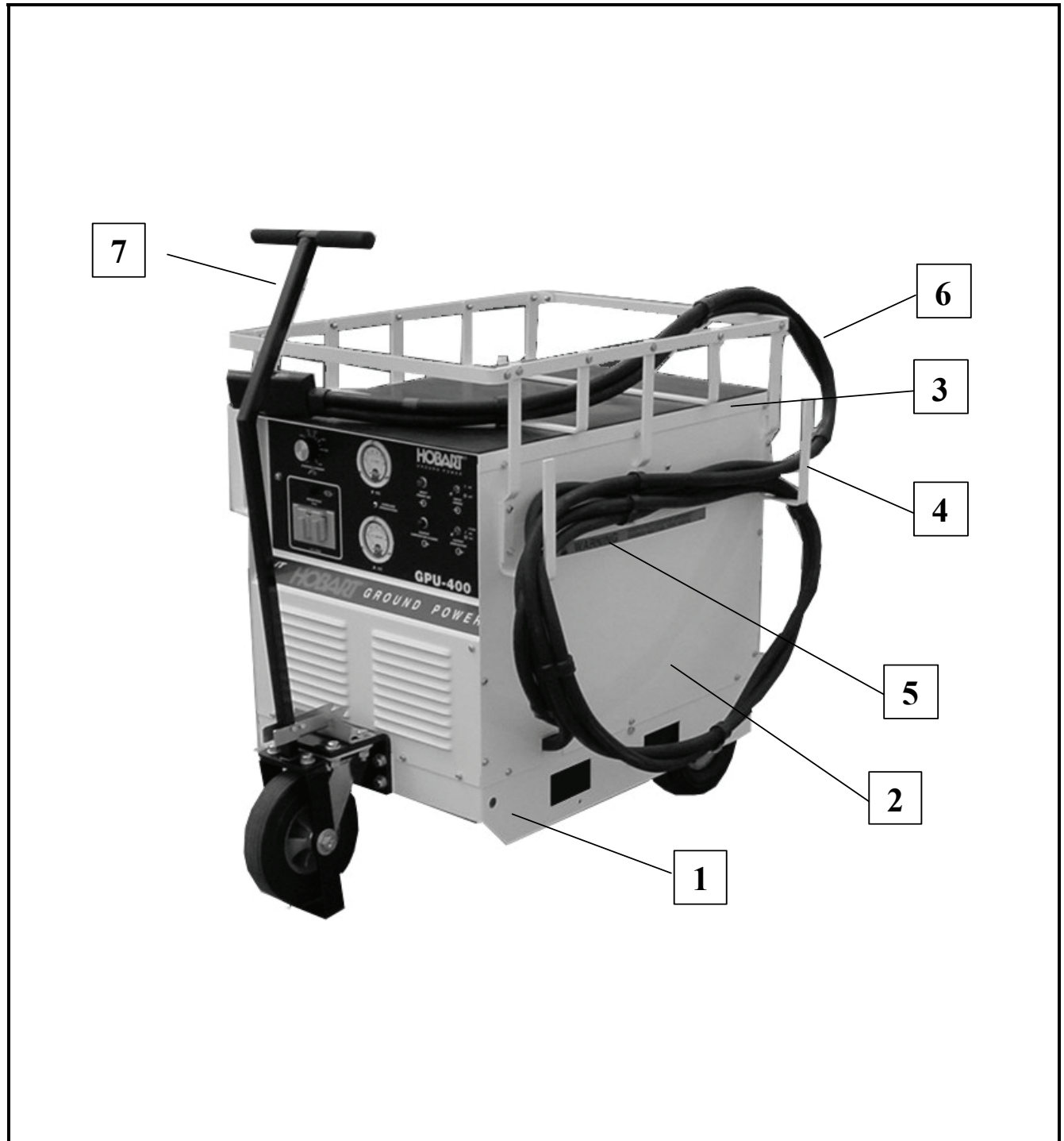
Final Assembly of GPU-400 Power Supply Figure 1
