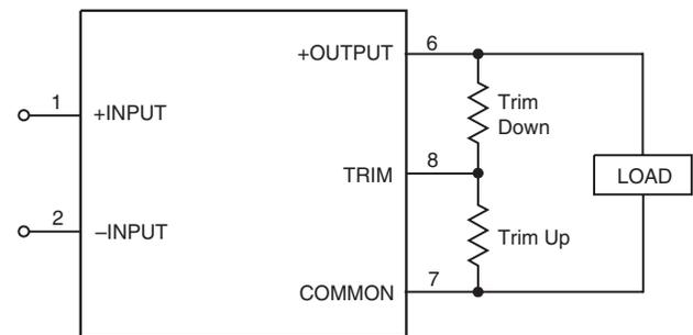
Figure 2b. Trim Connections Using Fixed Resistors
