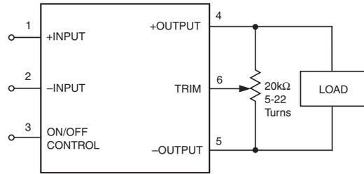
Figure 2. Trim Connections Using A Trim Pot
