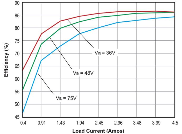
UEP-3.3/4500-D12 Efficiency vs. Line Voltage and Load Current
