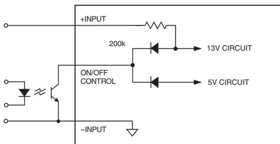
Figure 2. Driving the Positive Polarity On/Off Control Pin
