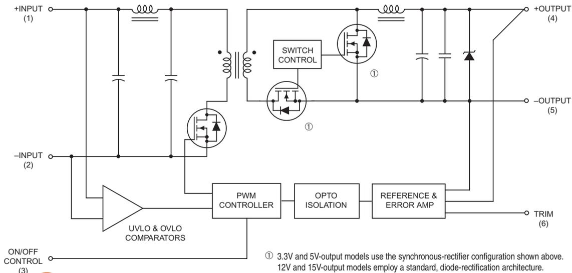
Figure 1. Simplified Schematic
