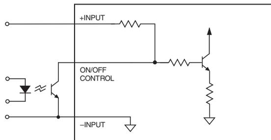
Figure 3. Driving the Negative Polarity On/Off Control Pin
