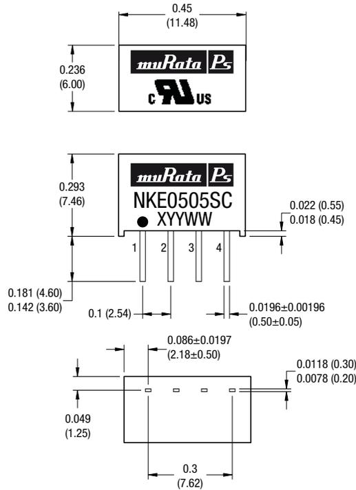
All dimensions in inches ±0.01 (mm ±0.25mm). All pins on a 0.1 (2.54) pitch and within ±0.01 (0.25) of true position.
