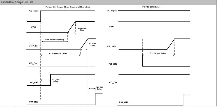
1. The turn-on delay after application of AC input within the operating range shall as defined in the following tables.
