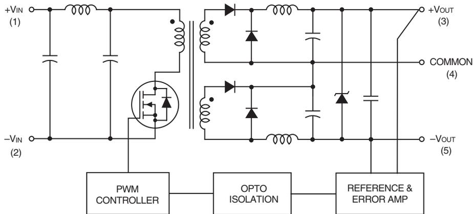
Figure 1. Simplified Schematic
