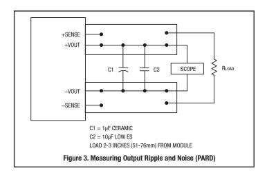
random deviations or PARD) may be reduced by adding filter elements such as multiple external capacitors. Be sure to calculate component temperature rise from reflected AC current dissipated inside capacitor ESR. Our Application Engineers can recommend potential solutions.
