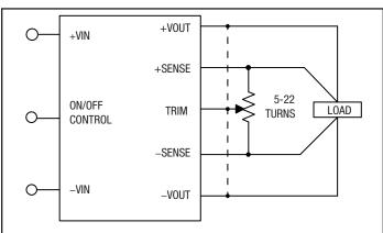
Figure 5. Trim adjustments using a trimpot; if sense is omitted, connect trim pin to either +output or -output.
