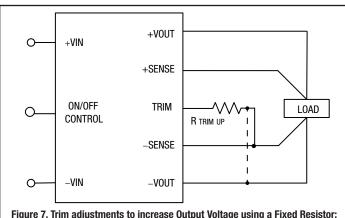
Figure 7. Trim adjustments to increase Output Voltage using a Fixed Resistor; if sense is omitted, connect trim pin to -output.
