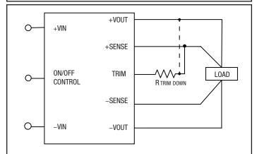
Figure 6. Trim adjustments to decrease Output Voltage using a Fixed Resistor; if sense is omitted, connect trim pin to +output.
