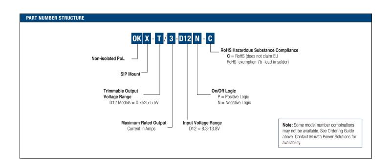
Adjustable 3-Amp SIP Non-Isolated DC/DC Converters
