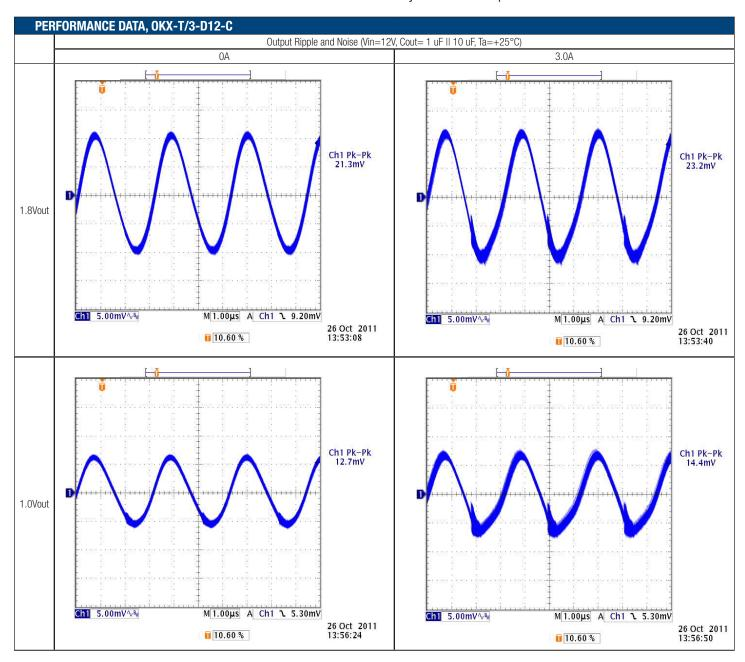
Adjustable 3-Amp SIP Non-Isolated DC/DC Converters
