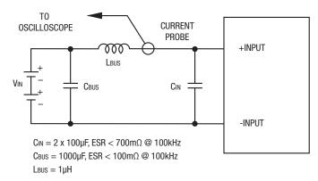
Figure 2. Measuring Input Ripple Current
