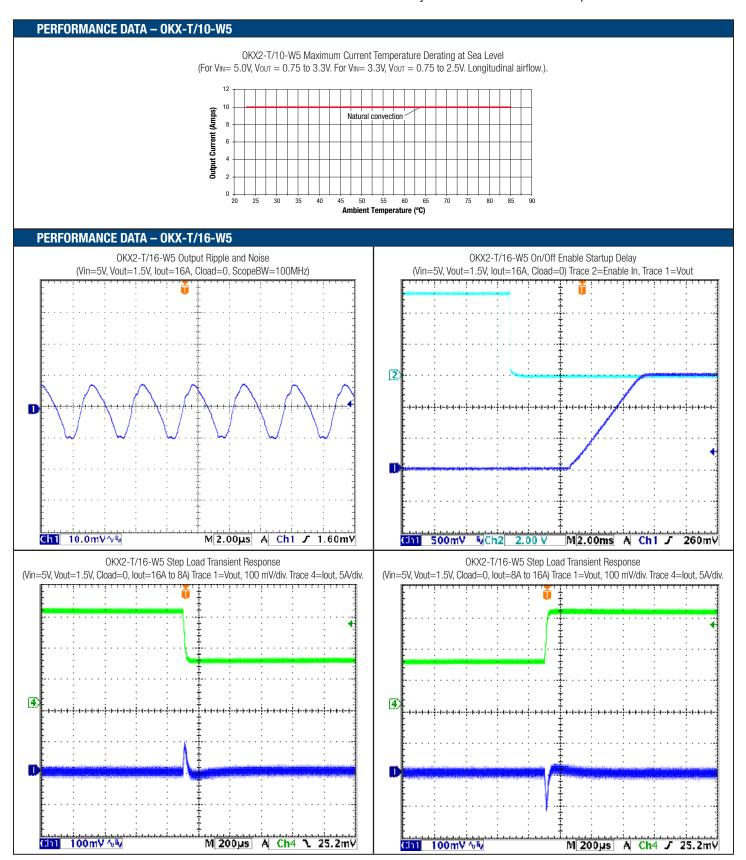
In this graphic data, 10 Amp models perform identically to 16 Amp models with the limitation of 10 Amps output.
