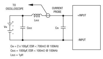
Figure 2: Measuring Input Ripple Current
