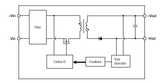
Figure 1. Simplified Block Diagram Typical topology is shown.
