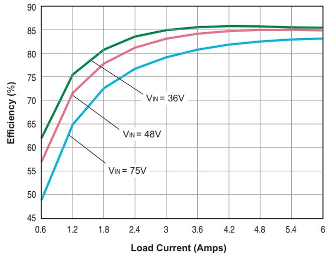
**UWR-1.5/6000-D48A Efficiency vs. Line and Load**
