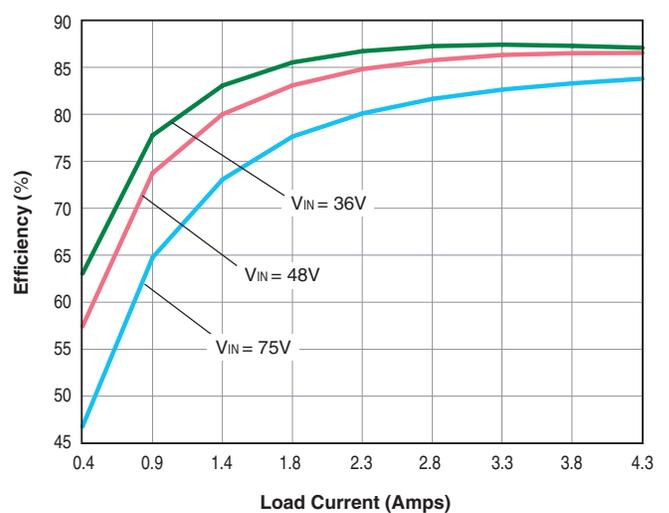
Single Output, High Density, 1" x 2" 6 Amp/15 Watt, 1.2-15V<sub>out</sub> DC/DC's
