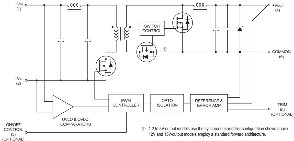
Figure 1. Simplified Schematic
