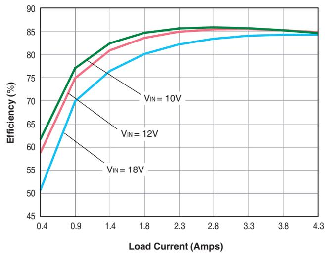
**UWR-2.5/6000-D24A Efficiency vs. Line and Load**
