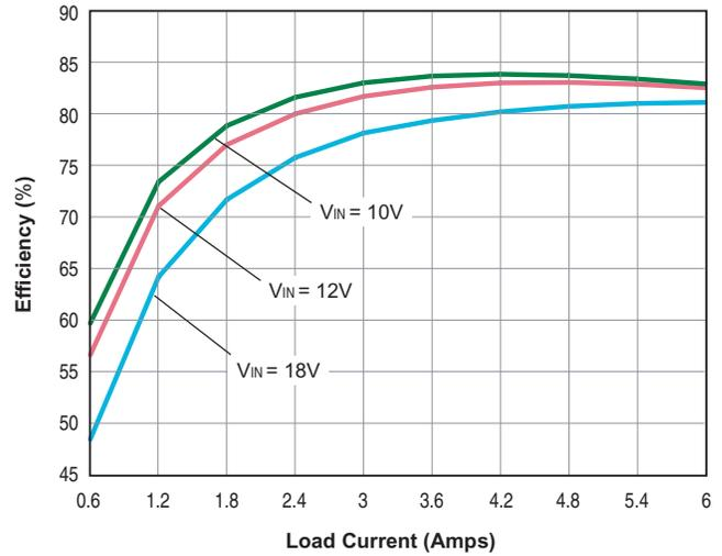
**UWR-1.5/6000-D24A Efficiency vs. Line and Load**
