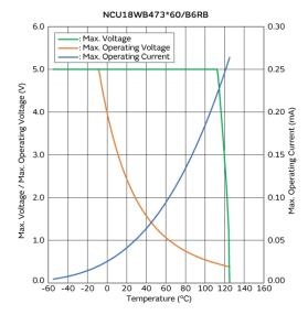
Max. Voltage, Max. Operating Voltage/Current **Reduction Curve**
