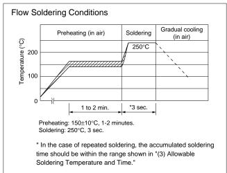
(5) There may be a risk of unexpected failures (tombstone, insufficient solder-wetting, etc.) in the mounting process caused by mounting conditions. Please make sure that this product is correctly mounted under the specified mounting conditions. (3) Allowable Soldering Temperature and Time(a) Solder within the temperature and time combinations, indicated by the slanted lines in the
