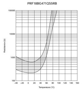
■ Resistance - Temperature Characteristics Range (Ref. Only) Tight Tolerance Type
