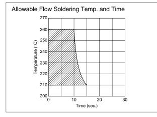
(4) Recommendable Temperature Profile for Soldering
