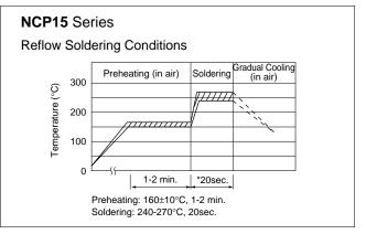
\* In the case of repeated soldering, the accumulated soldering time should be within the range shown in "2. Allowable Soldering Temperature and Time."
