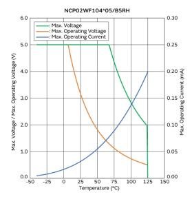
Max. Voltage, Max. Operating Voltage/Current Reduction Curve
