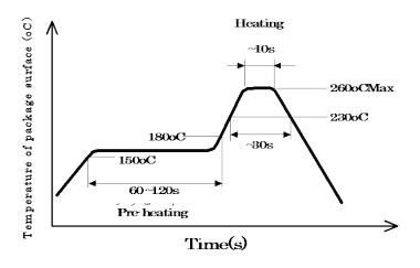
Times of reflow: 3 or less Hand soldering condition: 350+/-5°C, within 3 sec/each terminal
